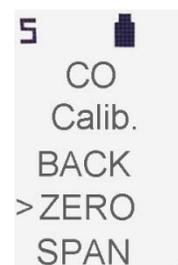
In order to perform a ZERO point calibration you need to have a reference gas with 0 ppm such as a scuba tank containing good air or just ambient air.
