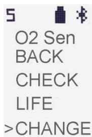
Please note that when you replace the Oxygen sensor while in stand-alone mode, Nitroxbuddy2 will automatically assign to the O2 sensor a lifetime of 12 months.
