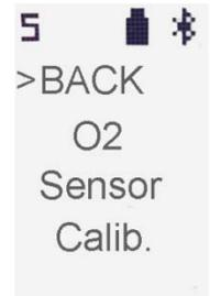
As indicated earlier, HOLD enters the sub-menu selected by the pointer while a PUSH moves to the next line down. In this specific case, HOLD will go back to the previous menu while PUSH will start the calibration of the Oxygen sensor.
